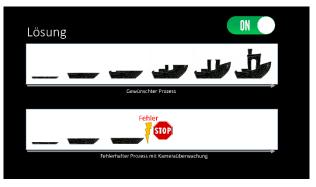
deviation, an error message appears and the process is aborted. This avoids unnecessary use of material and further printing errors and reduces unnecessary operation of the 3D printer.
